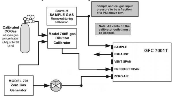
Figure 3-21: Pneumatic Connections – Option 50A: Zero/Span Calibration Valves
